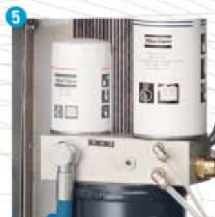
Oil filter & oil separator
