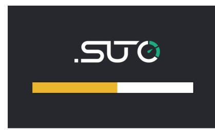
When the S 601 gets powered you will see the start up screen. The progress bar shows, that the sensors are configured and the device is running some initialization routines.
