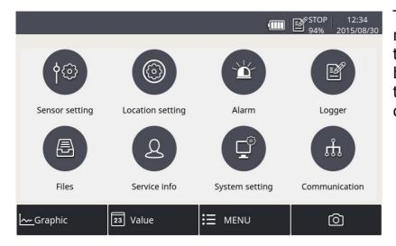
The user can get to the main menu by pressing the menu bar in the bottom bar. From here the user can get to different sub-menus.
