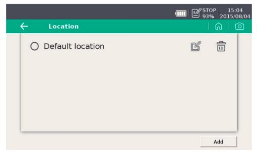
This function is used to assign the connected sensor and sub-displays (in case S 330 / 331 is a master device) into different locations (room1, room2 etc.)
