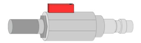
To check your point of measurement connect the purge filter test kit onto your measuring point first. Open the purge valve on the test kit and purge some air for a short period. Afterward check the filter in the test kit, if it shows high contamination of water, oil or dust. Should the filter be contaminated to high do not continue to measure with the S 601 as this may lead to serious damage. In case you are not sure, please contact the manufacturer.
