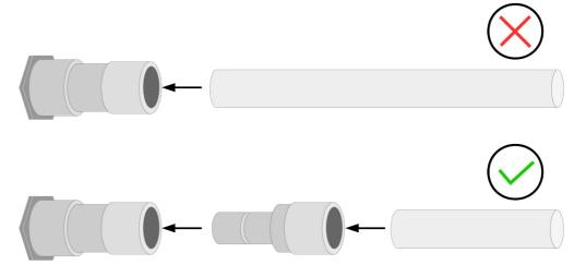
Using a quick connector more than once may lead to particle contamination which can affect the measurement. For this please use the included adapter plugs and keep them on your tubes.
