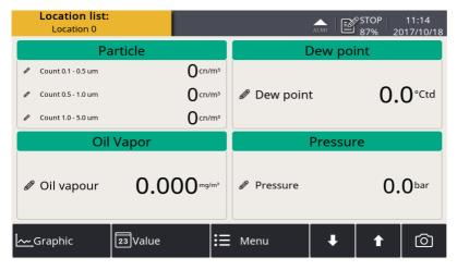
The user can switch to the value screen by pressing value in bottom bar. It will show the measured values in real time.
