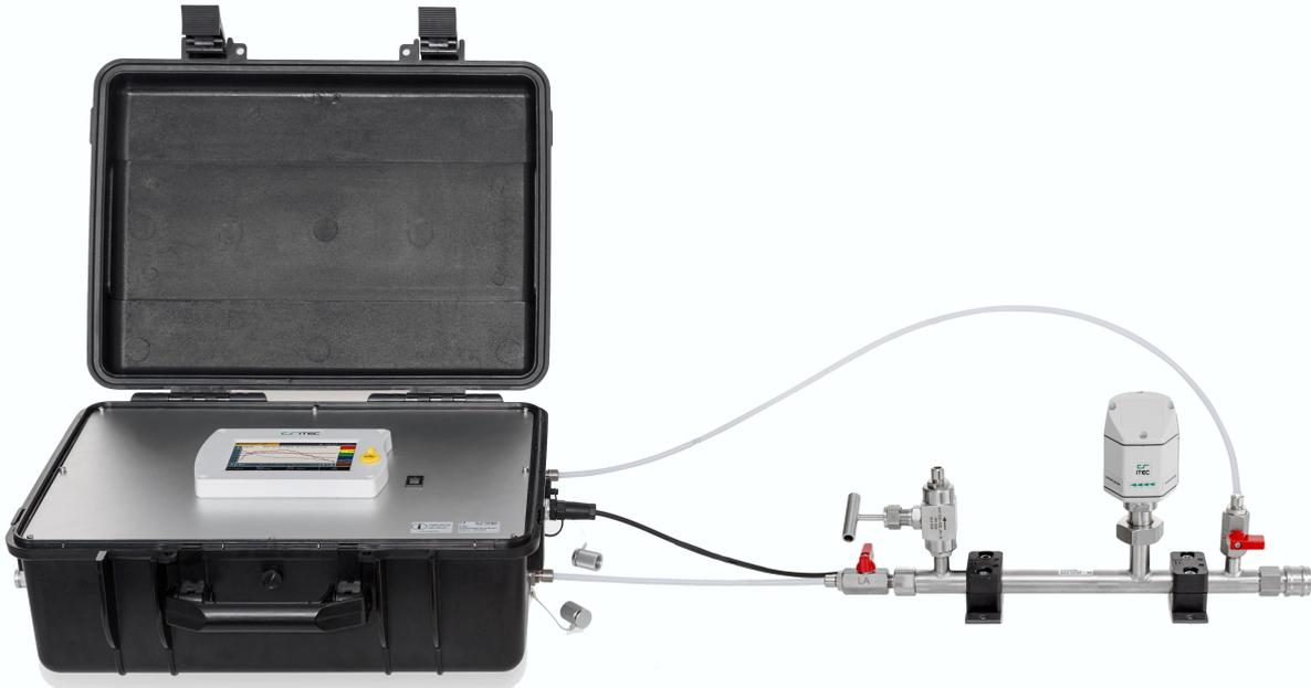
The picture above shows the setup together with the isokinetic sampling device connected to the S 600. Please connect the isokinetic sampling device using the teflon hose which came with the device. On the next page you will find a detailed description of the sampling device. Also you will find which outlets of the sampling device need to be connected to which input at the S 600.
