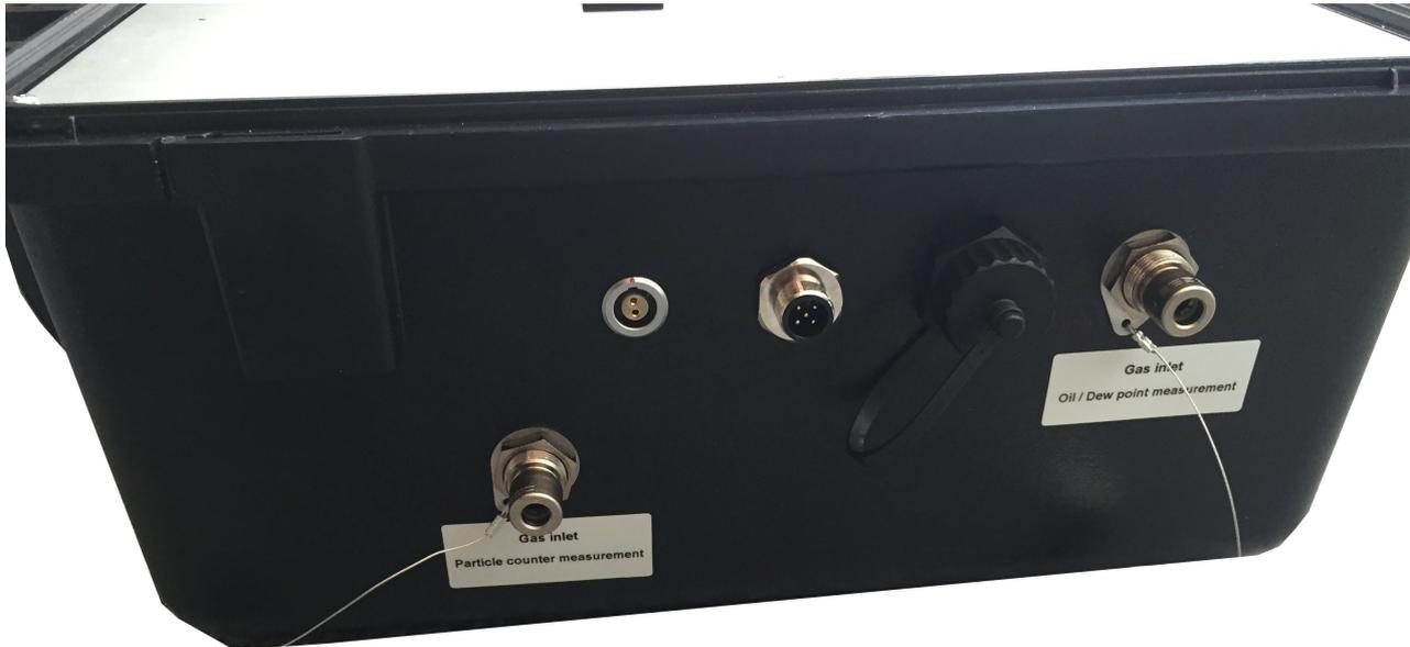
The S 600 offers two compressed air inputs on the right side of the housing. The inlets are shown on the picture above and are marked respectively to their functions: *Gas inlet Oil / Dew point measurement* and *Gas inlet Particle measurement*.
