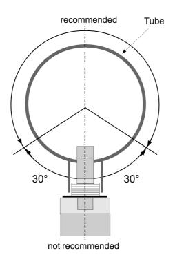
Please install the sensor only in the recommended area like you can see in the picture. A upside down installation is not permitted. Please consider that the distance to the vertical level must be >30°.
