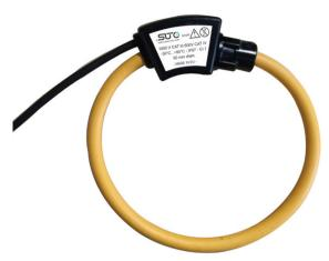
SUTO Miniflex 1000 current clamp sensor is an AC RMS current sensor composed of a flexible active part (Rogowski coil model) connected to a compact digital converter, capable of measuring the current carried on a power conductor up to a value of 1000 Aac.
