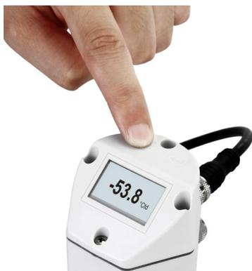
Alarm adjustment at dew point sensor
